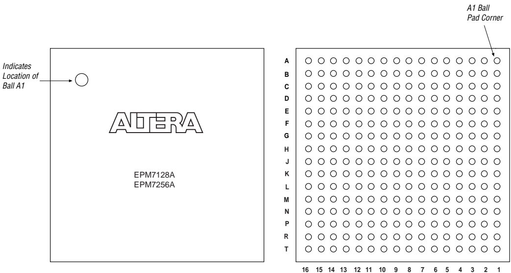
Figure 18. 256-Pin FineLine BGA Package Pin-Out Diagram
