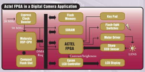
\*Actel's e-Appliance FPGAs combine low power consumption with high performance and capacity, enabling kernel hardware functions.
